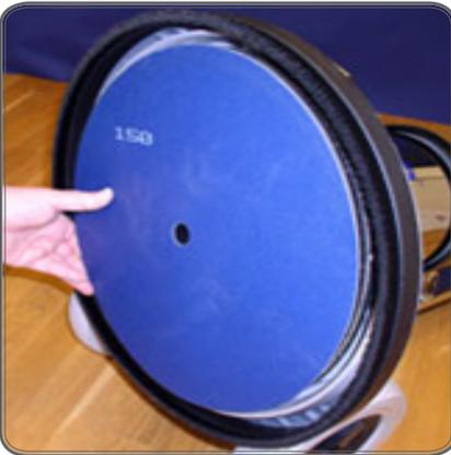
4) Insert and tighten the centre screw.
