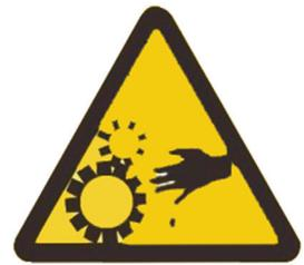
Hazard due to moving parts.
