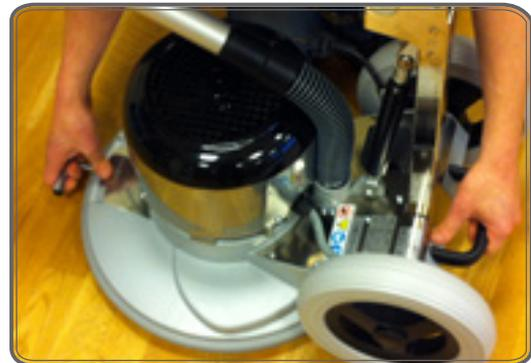
**NOTE! Always remove the dust skirt and the sanding disc before transportation!**
